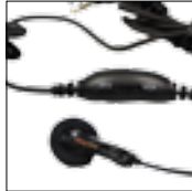
Mag One ear bud with in-line mic/PTT/VOX switch PMLN4442
