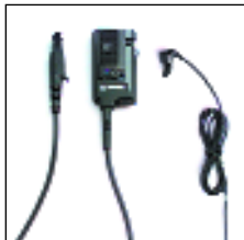
VOX/PTT Interface Module shown with Ear Microphone
